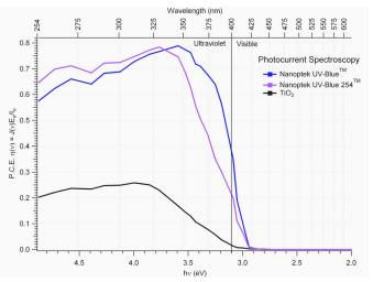
UV-Blue<sup>™</sup> is a robust thick film that is thermally grown onto and into a nano-structured titanium substrate. Our process is designed to work with economical "commercially pure" Grades 1 and 2 of titanium that are widely available as tubes, plates, or sheets. We also produce UV-Blue 254<sup>™</sup> that we tune for an improved response at the 254 nm wavelength of germicidal lamps used in water purification systems.
