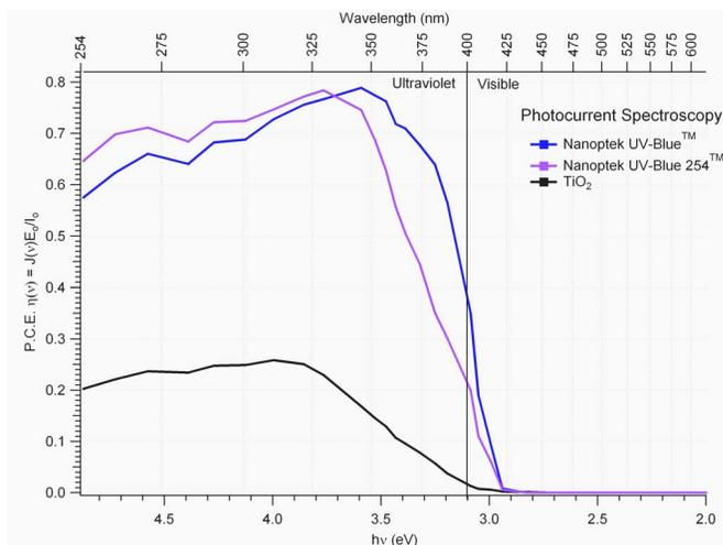
UV-Blue™ is a robust thick film that is thermally grown onto and into a nano-structured titanium substrate. Our process is designed to work with economical "commercially pure" Grades 1 and 2 of titanium that are widely available as tubes, plates, or sheets. We also produce UV-Blue 254™ that we tune for an improved response at the 254 nm wavelength of germicidal lamps used in water purification systems.
